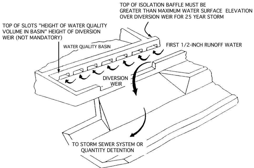
Figure 2: Examples of Isolation/Diversion Structure
