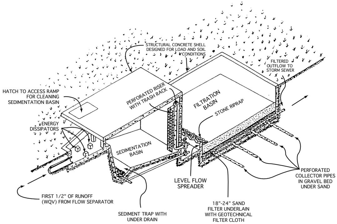
**Figure 3a: Austin Sand Filter with Full Sedimentation Protection**
