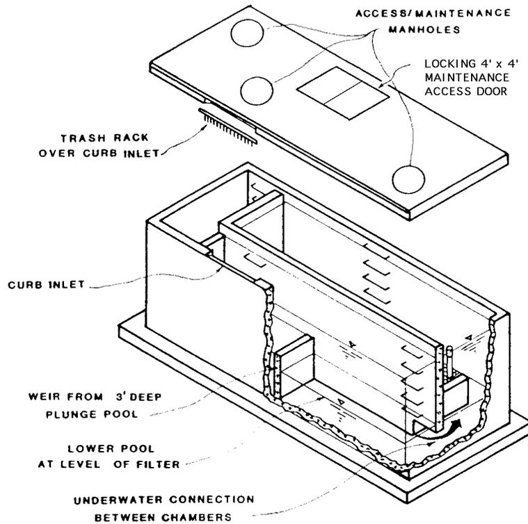
SEDIMENTATION CHAMBER CUTAWAY
