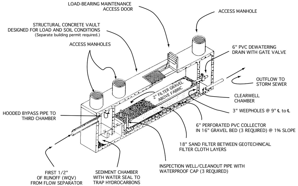
**Figure 10: Original D.C. Sand Filter (DCSF) System**
