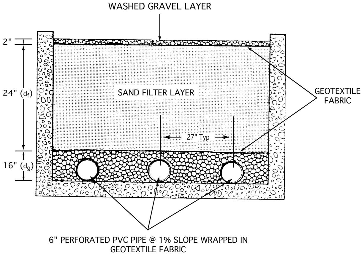
**Figure 12: Cross-Section of DCSF Filter**
