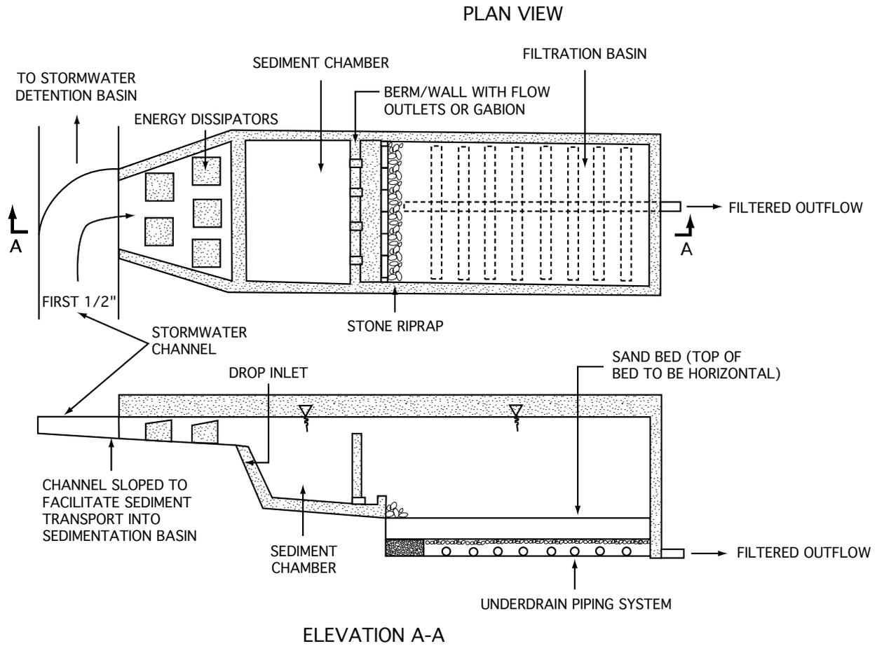
**Figure 9: Conceptual Partial Sedimentation - Filtration System**
