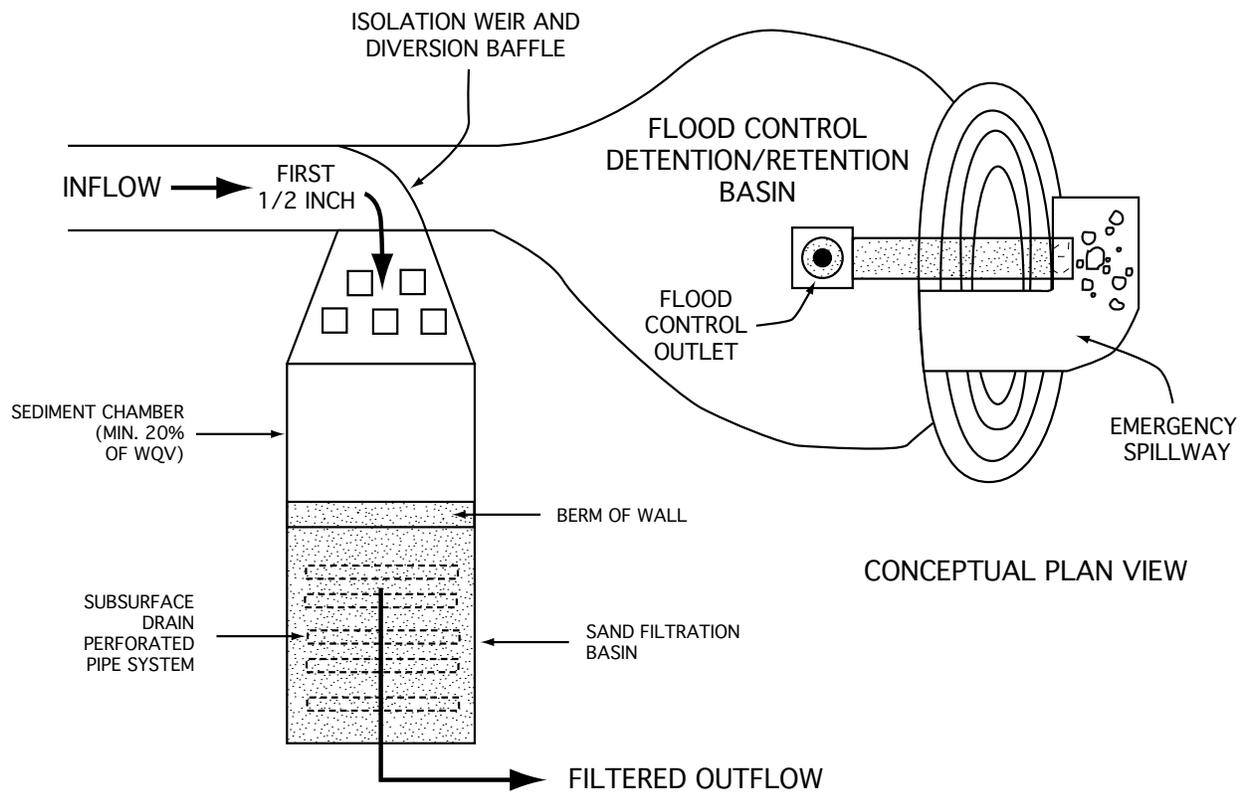
**Figure 7: Partial Sedimentation-Filtration (Plan View)**
