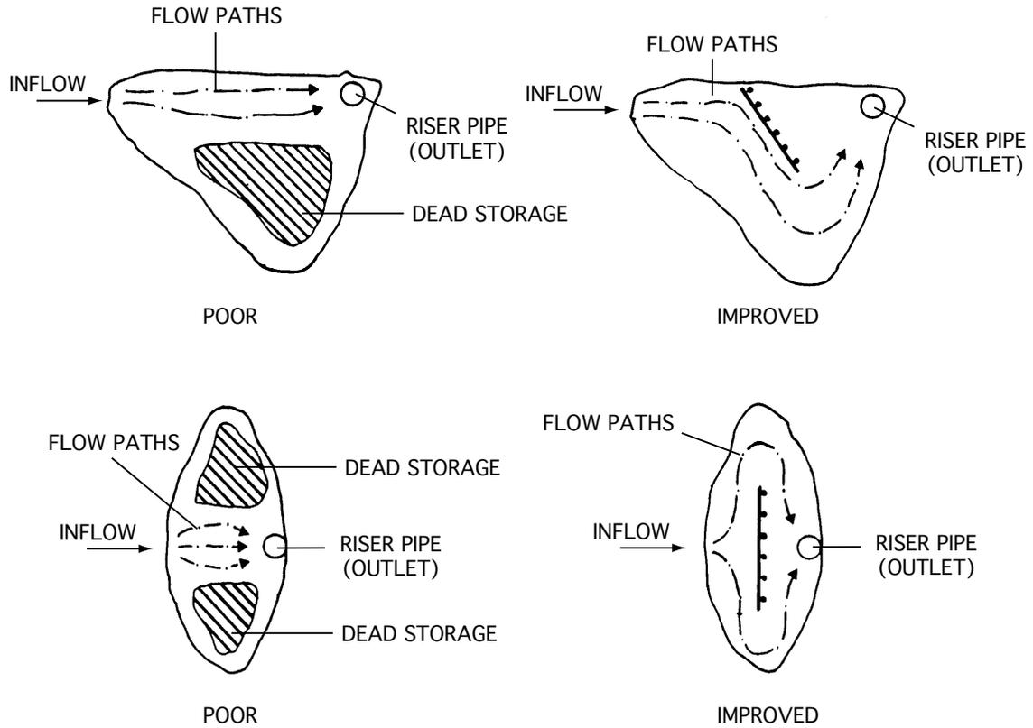
**Figure 4: Sedimentation Basin Baffles**
