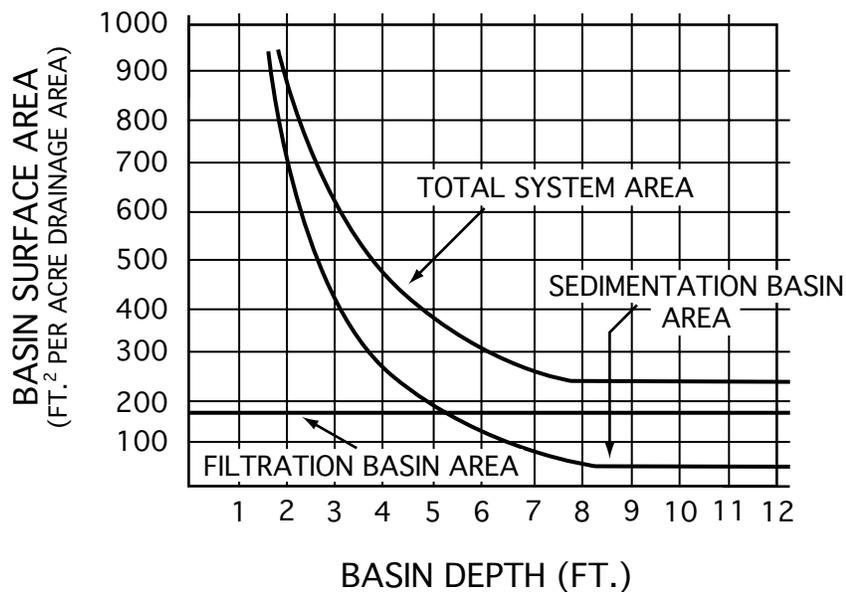
**Figure 8: Sedimentation/Filtration Basin Surface Areas**
