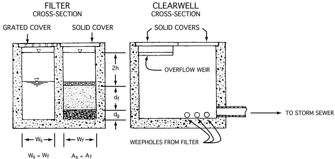
**Figure 15: Dimensional Relationships for Delaware Sand Filters**
