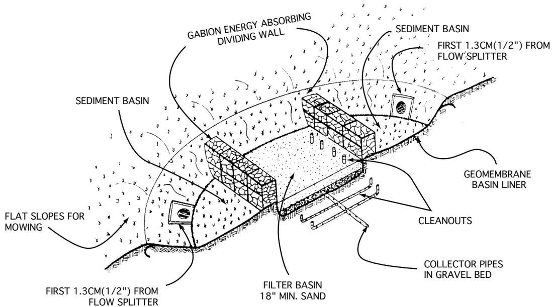
**Figure 3b: Austin Sand Filter with Partial Sedimentation Protection**
