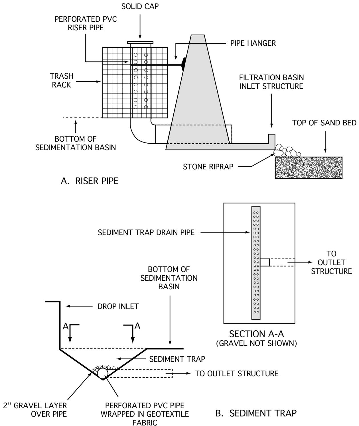
**Figure 5: Example Riser Pipe and Sediment Trap Details**
