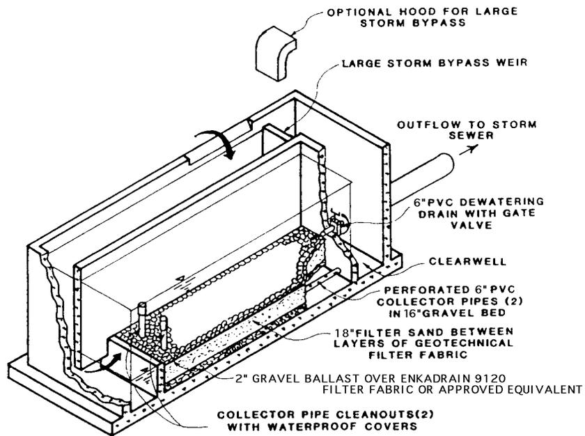
FILTER CHAMBER CUTAWAY
