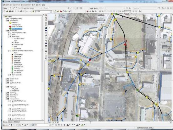
Mapping locations where sanitary and storm sewer lines cross to target areas where discharges could occur.
