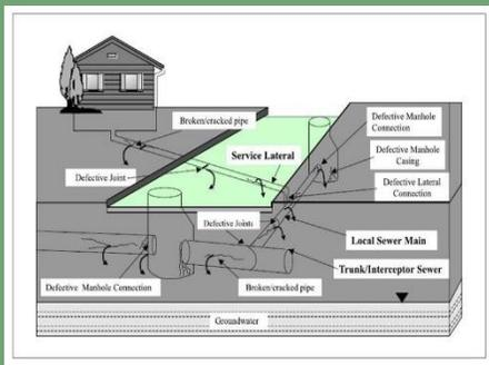
6. Schematic of sewage pipe exfiltration.
