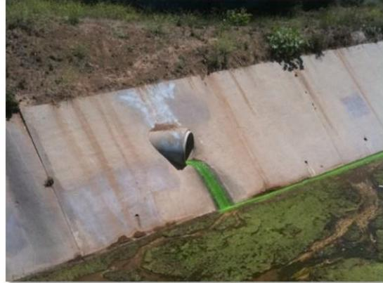
Fluorescent dye is introduced into the sewer network and suspected manholes are inspected to trace the flow through the network to locate the specific discharge.
