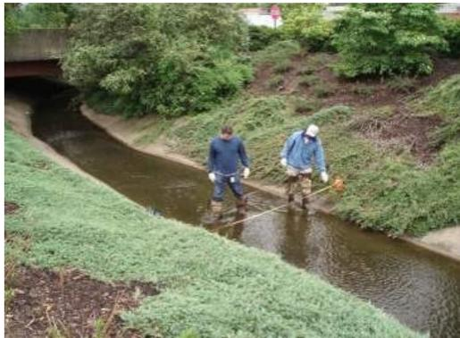
Walk streams in the watershed to inventory all outfalls in the MS4, visually assess and collect samples to identify possible high nutrient discharges.
