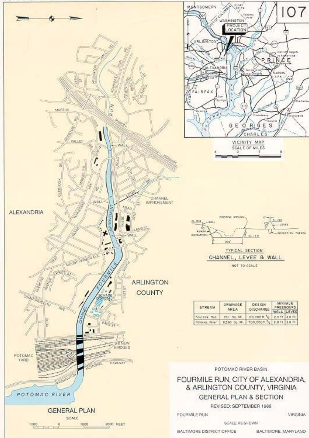
Figure 2 – Local Flood Protection Project General Plan, 1988
