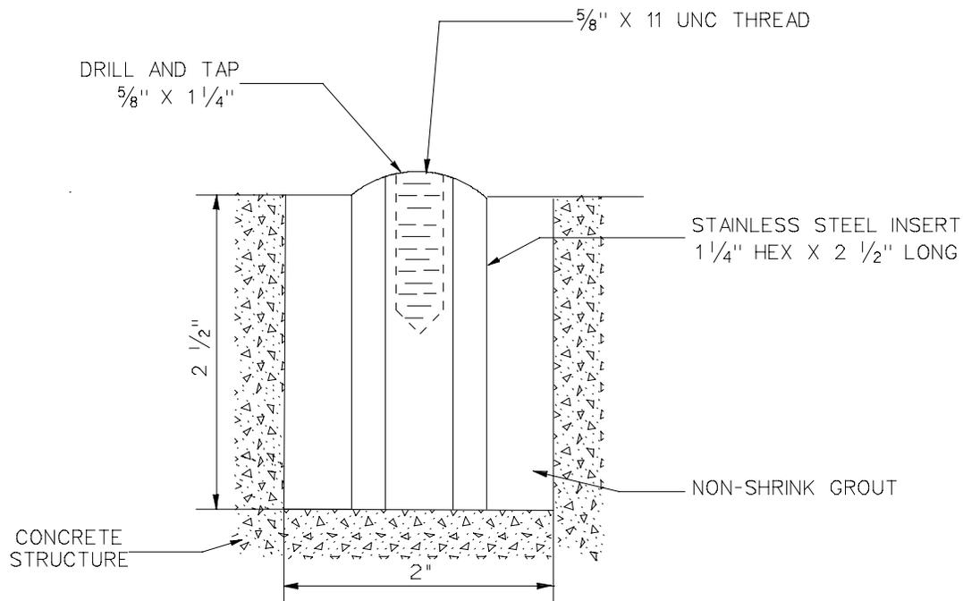
Figure 4-4. Structure insert
