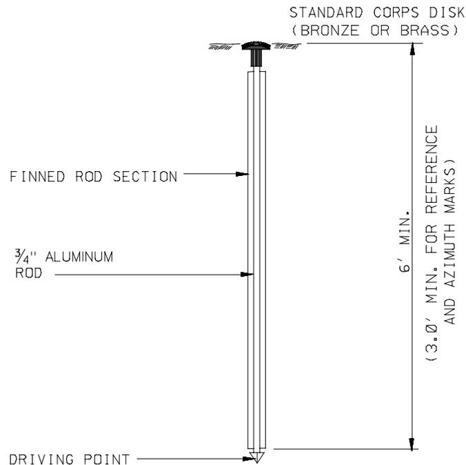
USE FOR HORIZONTAL, BOUNDARY, REFERENCE AND AZIMUTH CONTROL
