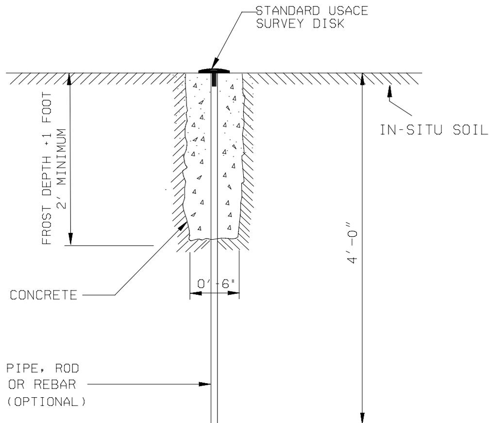
Figure 3-8. Type G monument - disk in cast-in-place concrete
